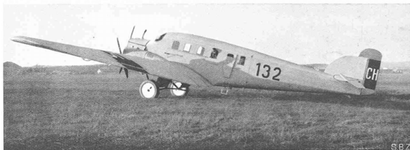
Abb. 14. Junkers G 24, 3 \times 280/310 PS, SpW 28,5 m, L 15,2 m. G = 4300 + 2200 kg. 200 km/h, 9 Passagiere. Deutsche Lufthansa. Zürich-Stuttgart-Berlin, Genf-Basel-Frankfurt-Hamburg.
